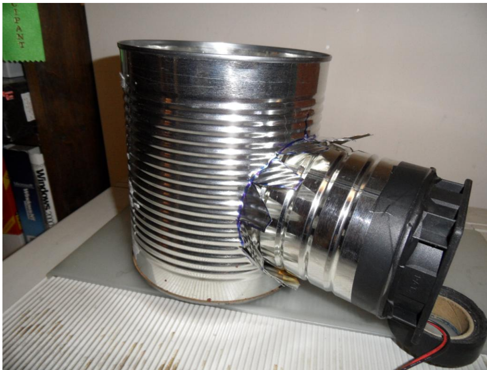
Figure 3: Attaching the fan-can to the larger can
