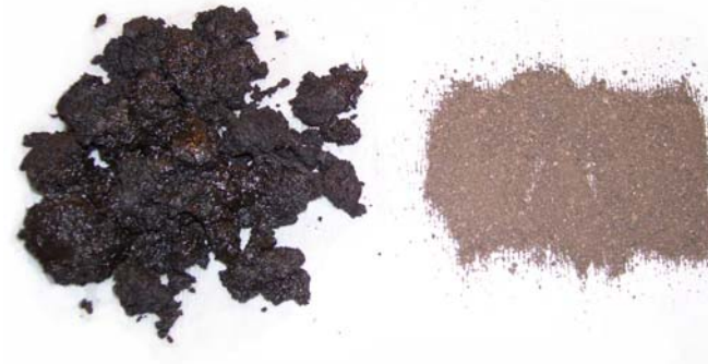
Oily waste sludge reduced to harmless hydrocarbon free ash
