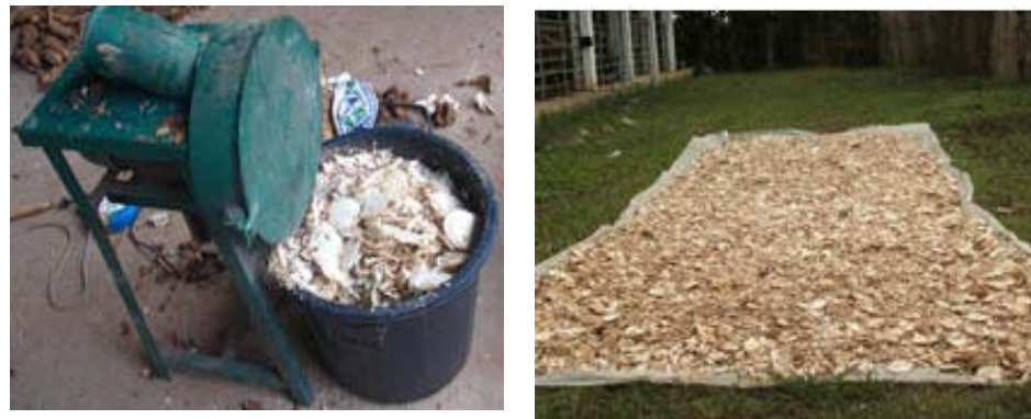
Photo 1: Chopping the cassava root by machine
