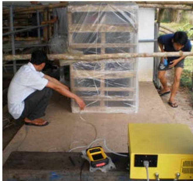
Photo 5: Wooden crates enclosed in plastic used to house the cattle during the 5 minute period of adaptation/measurement using the GASMET infra-red analyser.
