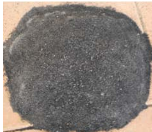
Photo 2: Biochar from updraft gasifier stove
