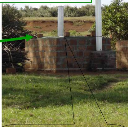
This innovative "low-cost retort kiln" (adam-retort) needs just about halve of the wood for producing the same amount of charcoal from wood or other biomass (briquetts & ECO CHARCOAL).
