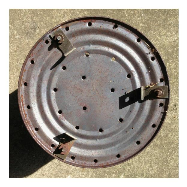
The primary air holes in the bottom of the iCan reactor can. These holes were made with a 5/32s drill bit.
