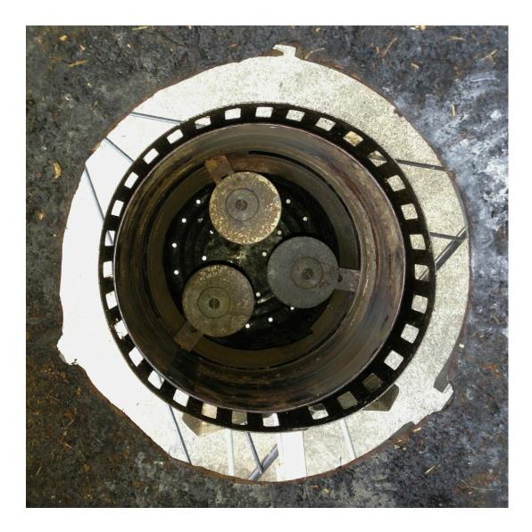
A view down through the aperture in the bottom of the Weber kettle into an empty iCan system. The reactor can and the draft can are sitting inside the outer shell.
