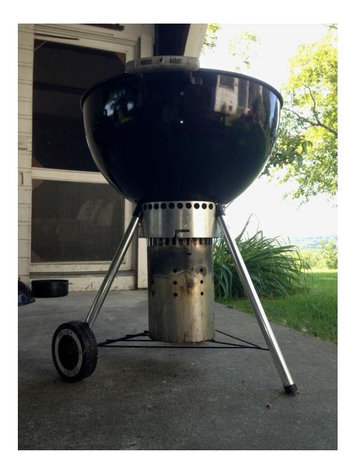
The outer shell, shown here, acts to protect the cans from accidental tipping as well as to prevent wind gusts from blowing out the gas fire. The outer shell shown here is made from a Weber charcoal starter with its inner basket removed. It could also be made from a section of stove pipe cut to size.
